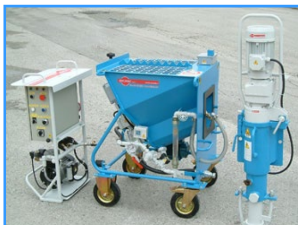
CK 20 disassembled in 3 parts, easy to carry.
