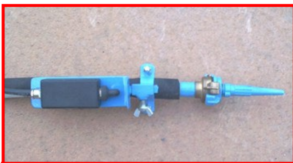
Filling gun for joints with wired 24 V remote control
